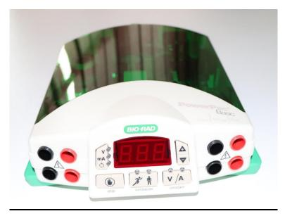
The PowerPac<sup>TM</sup> Basic power supply is recommended for basic applications such as submerged horizontal and mini vertical gel electrophoresis.
