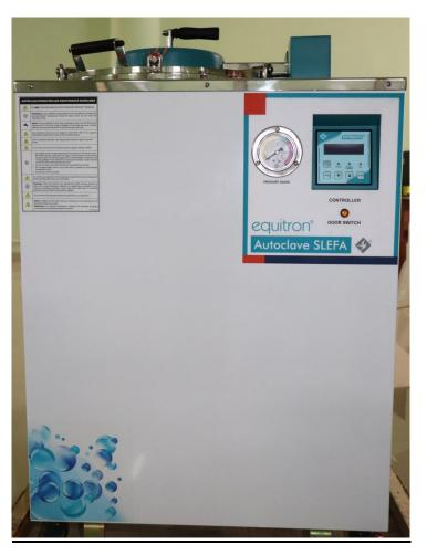
Autoclaves provide a physical method for disinfection and sterilization with a combination of high temperature, steam, pressure and time in order to kill infectious microorganisms and spores. They are also used to decontaminate certain biological waste and sterilize media, instruments, lab ware, medical waste that might contain bacteria, viruses and other biological materials that are recommended to be inactivated by autoclaving before disposal.
