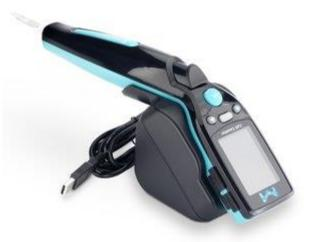
The Scepter Cell Counter is used to perform a fast and convenient cell counts in an easy to use format. This instrument is used in sampling process where it reveals data on cell concentration, average diameter, average volume and histogram displaying population information on your culture within 30-40 seconds. The time to perform the cell counting experiment has been reduced from approx. 10-15 minutes in conventional cell counting systems to less than 30 seconds by the
