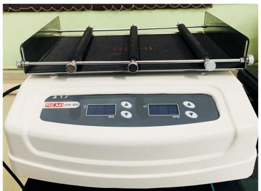
Mini rotator shakers are used for gentle mixing of samples, solvents, reaction mixtures, formulations and test preparations in test tubes, ELISA plates, mixing plates & glass vessels of different capacities. These shakers are used in pathology, microbiology, chemistry, molecular biology & biotechnology to develop a uniform mixture of solutions, reactants. Speed Range 80-180 RPM with 0-15 minutes timer.
