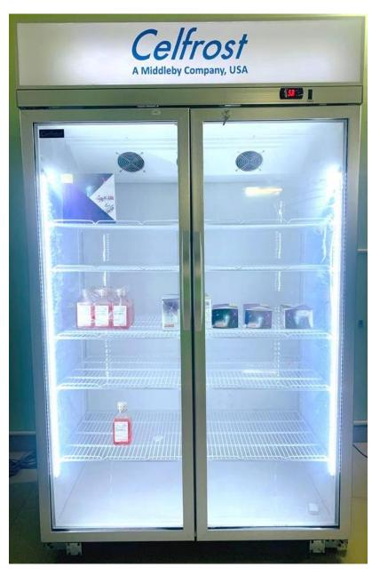
These refrigerators are used for maintain a cold storage conditions for samples, chemicals specified to be stored at 1-8 °C.
