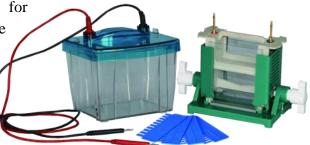
electrophoresis can be transferred to the membranes using the attached blotting assembly.
